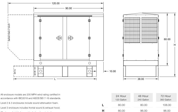
\*Enclosure height does not include exhaust stack.
